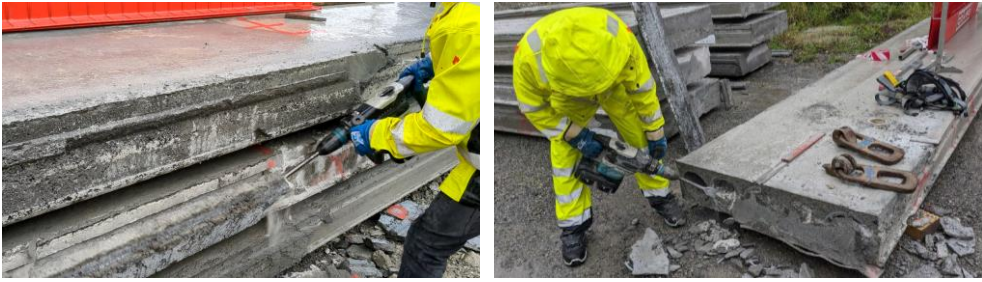
Fig. 7 Removal of grouting concrete from the longitudinal side of a HCS, where adhesion-reducing products were applied (left) and from a reference area at the short end of the HCS (right).
